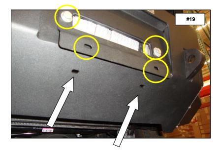
If installing a winch, attach the license plate directly to the (2) obround holes in the lower face of the bumper shell using the supplied  $\frac{1}{4}$ " bolts and nuts, (Photo 18).
