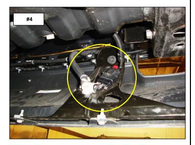
**Step-4** On each side of the vehicle, remove the bolt securing the outer bumper support bar to the bumper and loosen the (2) bolts securing the opposite end of the support bar to the frame body mount bracket, (Photo 5).
