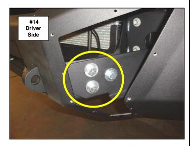
**Step-6** Align the holes and attach each factory bumper support bar to each of the bumper shell support brackets using (1)  $\frac{1}{2}$ " x 1  $\frac{1}{2}$ " hex bolt, (2)  $\frac{1}{2}$ " flat washers, (1)  $\frac{1}{2}$ " lock washer and (1)  $\frac{1}{2}$ " hex nut, (Photo 15).
