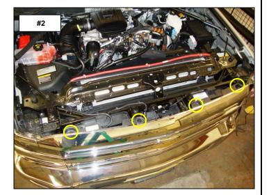
**Step-3** Working from side to side gently pull outward to unsnap the clips and remove the grille, (Photo 3).
