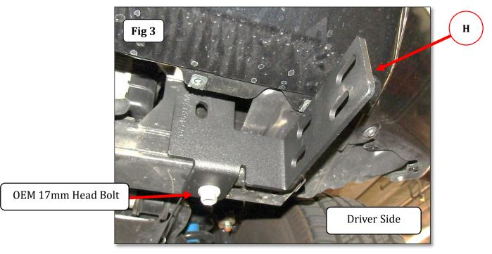
**Step-4** Align the holes and attach (1) auxiliary brackets and the driver side mounting bracket to the face of the frame using (1)  $\frac{1}{2}$ " x 4  $\frac{1}{2}$ " hex bolt, (2)  $\frac{1}{2}$ " flat washers, (1)  $\frac{1}{2}$ " lock washer and (1)  $\frac{1}{2}$ " hex nut., (Fig 4). Leave the nut and bolt loose for final adjustment. Repeat step 3 & 4 for the passenger side.
