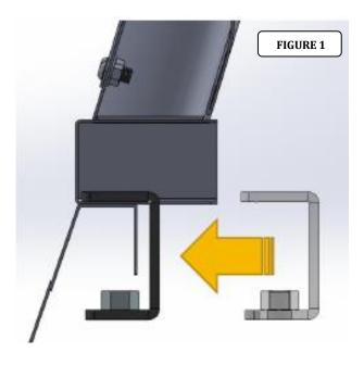
**Step-2** Place the auxiliary bracket underneath the bed cargo frame. Make sure the bracket surface contacts completely with the bed cargo frame (FIGURE 2).
