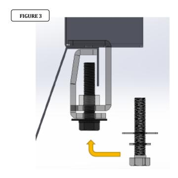
**Step-4** Use (2) sets of bracket per side. Align the Sport Bar 3.0 with the vehicle and tighten all bolts securing the Sport Bar 3.0 to the brackets. Repeat the above steps to install the passenger side brackets. Remember to check and retighten the nuts and bolts every six months.
