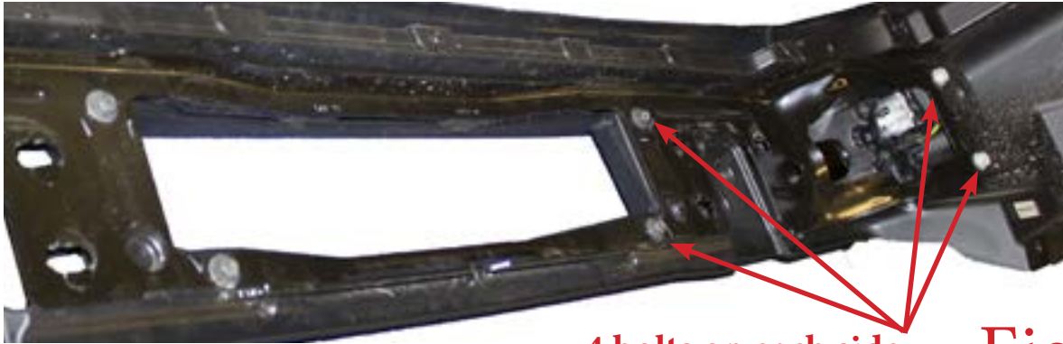
4 bolts on each side
