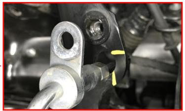
Remove brake line from factory mounting area.
