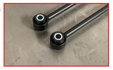
Use a fair amount of grease on the inside of the bushing and press the M10 crush sleeve into the bushing.
