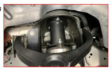
Swing the lower control arm up and install the factory lower strut bolt through the lower control arm.
