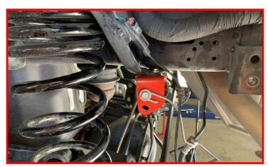
Install the ABS retaining clip into the driver rear brake line bracket in the bottom hole. Tighten the bracket at this time.
