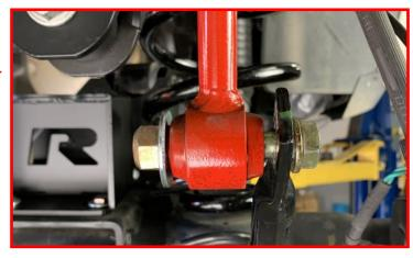
Note: Ensure the fender washer is installed on the bushing side.
