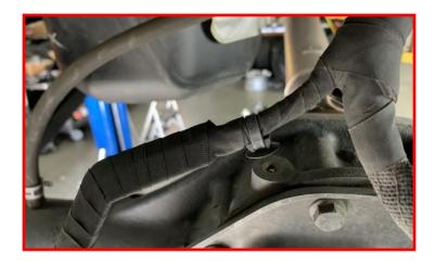
Install the harness retaining clip the stud on the rear differential cover.
