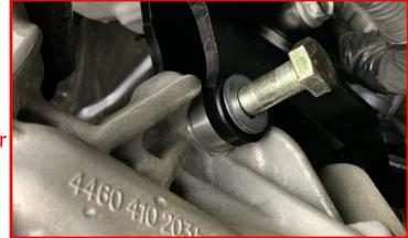
Install the (3) factory mounting bolts through the rear differential drop bracket and into the differential.
