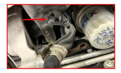
With an appropriate jack stand, support the front differential and remove the (2) driver side differential mounting bolts. Retain the factory hardware.
