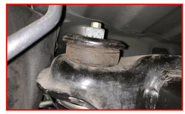
Loosen but do not remove the upper and lower trailing arm hardware.
