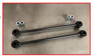
Use a fair amount of grease on the inside of the bushing and press the M12 crush sleeve into the bushing.
