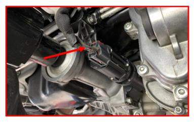
Remove the harness retaining clip from the retaining bracket attached to the differential mount.
