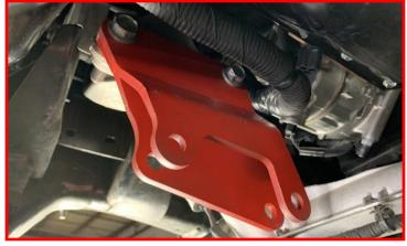
Install the passenger side front differential drop onto factory differential mounting point using the factory mounting bolts. Do not tighten at this time.
