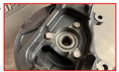
Install the completed knuckle assembly to the lower ball joint while guiding the CV axle through the hub.
