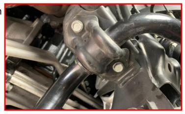
Remove the lower sway bar end link from the lower control arm. Remove sway bar from the vehicle and retain factory hardware.
