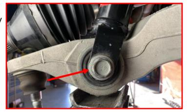
Swing lower control arm down and out of the way. Remove the (3) top strut nuts and carefully remove the strut from the vehicle.
