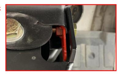
Install the track bar into the track bar bracket using the factory hardware. Do not tighten at this time.
