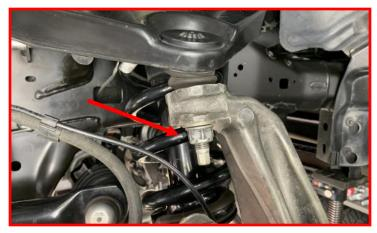
Loosen the upper control arm bolts located inside strut tower.
