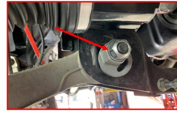
Remove the lower control arm from the frame. Be sure to retain factory alignment cam bolts, cams and nuts.
