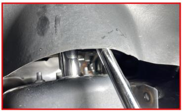
Remove the outer tie rod end nut.
