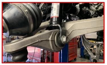
With the strut installed, use the supplied cable ties to secure the air line to the steel portion of the brake line.
