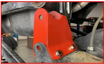
Install the supplied M16 bolt, locking nut and washers. Do not tighten at this time.
