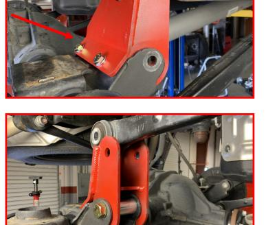
Install the supplied M8 bolt and washer through the upper control arm bracket and into the axle. Do not tighten at this time.
