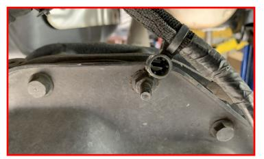
Support the axle with a suitable jack. Remove the lower shock bolt.
