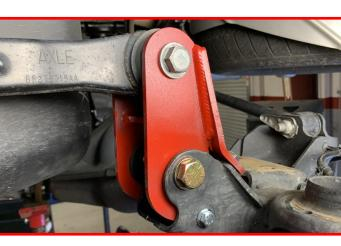
Attach the track bar bracket support tab to the factory track bar mount using the track bar bracket nut plate, the supplied M12 x 35mm bolt and washers and tread locker. Tighten all mounting hardware at this time.
