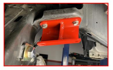
Install sway bar using the supplied M10 x 25mm bolts, washers and nuts hardware.
