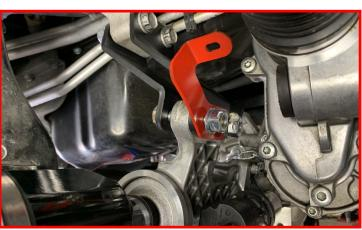
Install the top harness retaining clip into the shift solenoid harness bracket.
