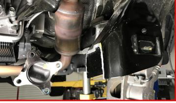
\*\*\*Parts shown in red for picture clarification only\*\*\* Install the driver side differential drops
