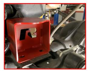
On the driver side only, Install the bump stop nut plate.
