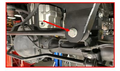
Ensure the welds that bond the bag mount to the axle housing do not rise above the mounting surface. If necessary, grind this weld flush and use paint or another type of sealer to protect against corrosion.
