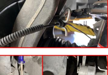
Remove the ride height sensor link from the control arm using a small pry bar or similar tool.
