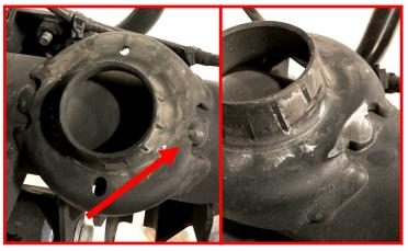
Install the air bag spacer using the  $1/4-20 \times 1''$  bolts, washers, and lock nuts. Orient the oval mounting hole toward the front of the vehicle.
