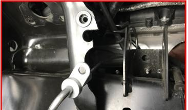
Using care, carefully pull down on the brake line. While pulling the brake line down into place you'll need to rotate the bulkhead fitting so the hardline is aimed toward the rear on the vehicle.
