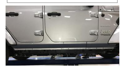
**Step 3.** Carefully raise step up into position and align the brackets with the factory mounting points with the horizontal part of the bracket on the outside of the pinch weld.
