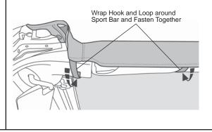
Wrap Hook and Loop around Sport Bar and Fasten Together
