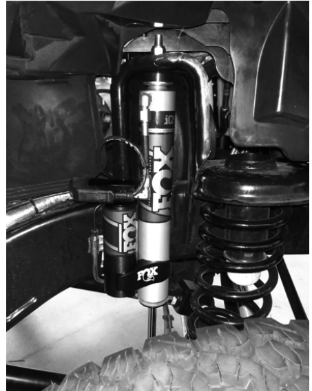
Fig. 17 Right Front (RF) IQS Shock Installed
