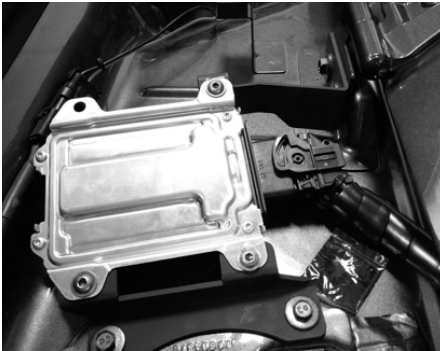
Fig. 12 ECU and Harness Secured, Connector Lever Perpendicular to Connector Face
