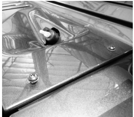
Fig. 4 Left Side Top Cowl Panel Bolts
