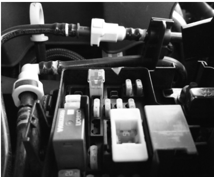
Fig. 13 Fuse Box Notch for Ignition Switch Wire Routing Shown
