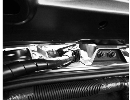
Fig. 10 ECU and Harness View from Engine Bay (Hood Lifted Up)
