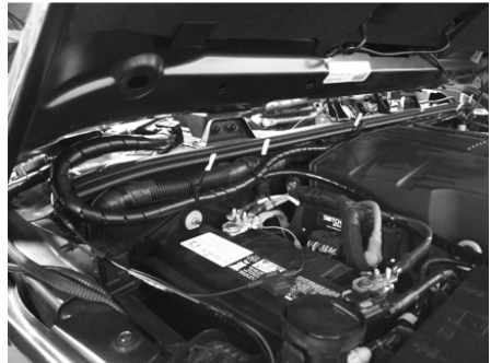
Fig. 14 Wire Harness Positioned Around Passenger Side of Hood Seal
