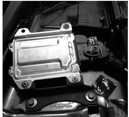
Fig. 11 ECU Connector Lever Parallel to Connector Face
