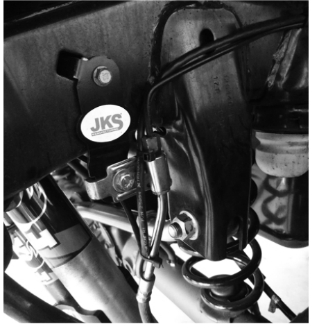
Fig. 20 RR Cable Routing Between The Right Rear Shock And The Rear Axle Track Bar
