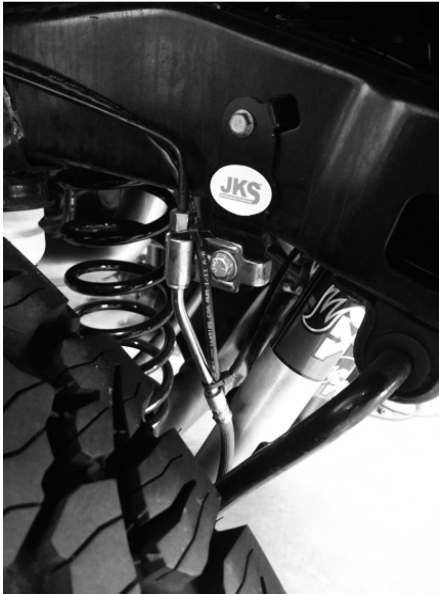
Fig. 28 LR Cable Routing Between The Left Rear Shock And The Rear Axle Track Bar.
