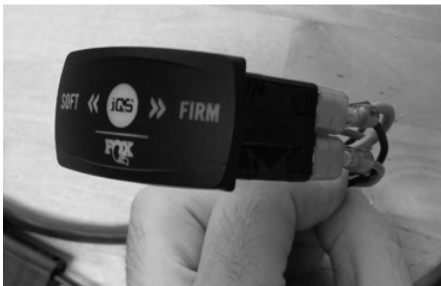
Fig. 32 Horizontal Layout iQS Switch: Firm Setting Aligned with Red Quick Connect Terminals on Right
