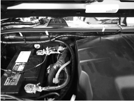
Fig. 15 RF (Right Front) and RR (Right Rear) Engine Bay Routing
