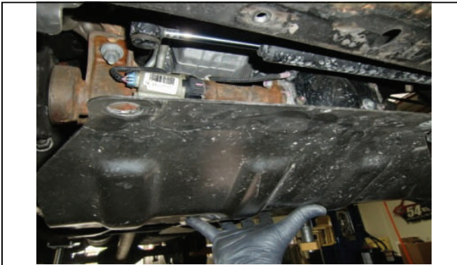
Remove skid plate bolts and skid plate
