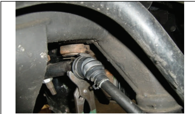
Loosen and remove inner/outer tie rod from center link.
