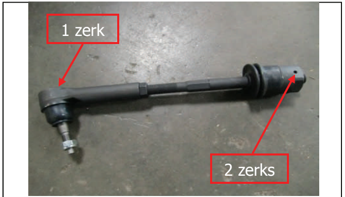
Locate new assembled HD steering kit and install zerk fittings
