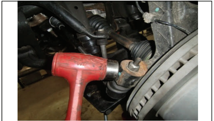
Disconnect outer tie rod nut and strike spindle to disconnect.
