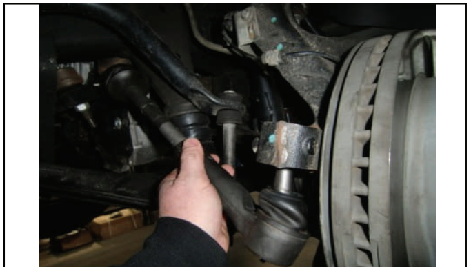
Attach outer tie rod to spindle and tighten
