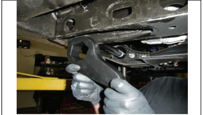
Install new torsion key and slide bar into position
