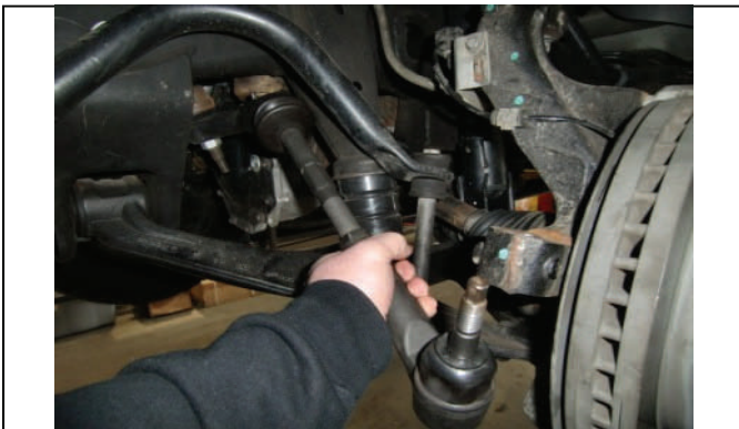
Install new steering assembly on center link
