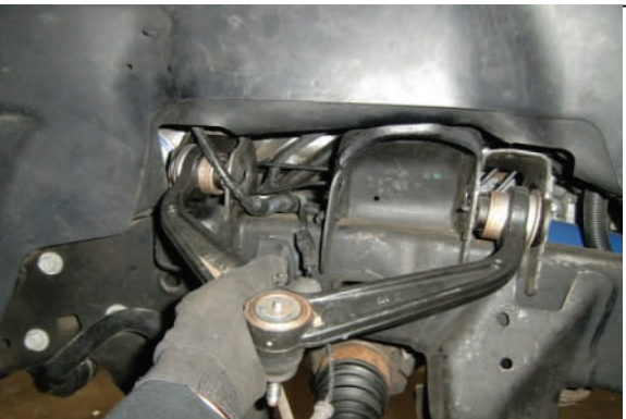
Remove upper control arm from frame pockets
