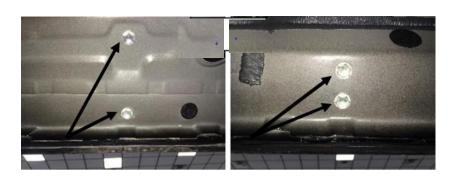
**Step 3:** Position step up to the body of the vehicle and align the brackets up with the factory mounting locations.
