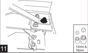
For all other Models: Using 19mm socket, tighten bolt to 35 ft-lbs. Tighten M8 screw from step 9 to 16 ft-lbs.
