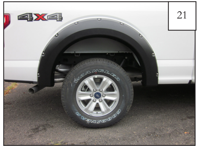
Completed rear flare installation.
