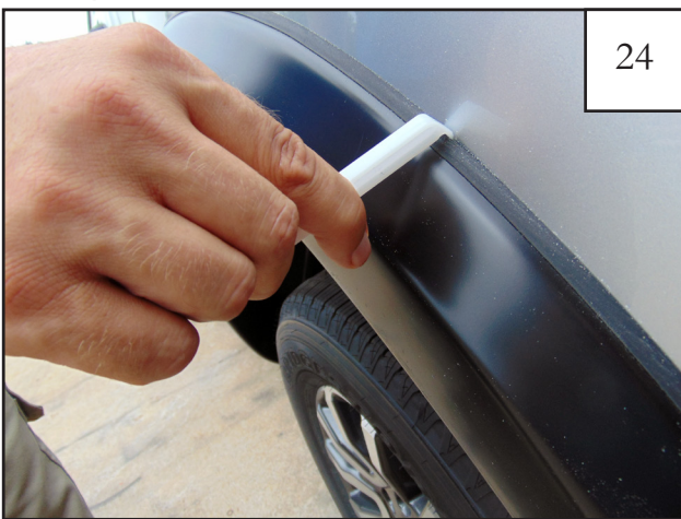
Using supplied Edge Trim Tool (ET1-0002), seat edge trim against vehicle by hooking curved end under edge trim at one end of flare. Next, slide around outer edge of flare to the other end.
