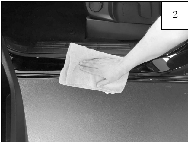
Open vehicle door. Clean all dirt and debris from vehicle then use supplied alcohol wipe where part will be. NOTE: Temperature should be at least 60°F for proper tape adhesion.
