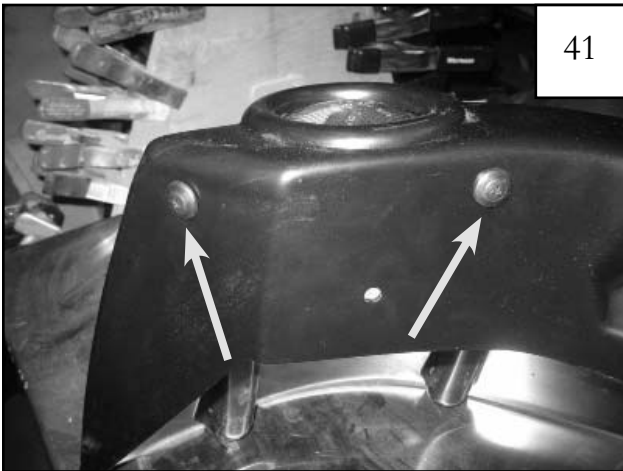
Install supplied Plastic Phillips Head Tuf-Loks (2 places). Use a pushing-twisting motion to install. Gently pull tab to peel tape liner from 1/2" tape and press in to place.
