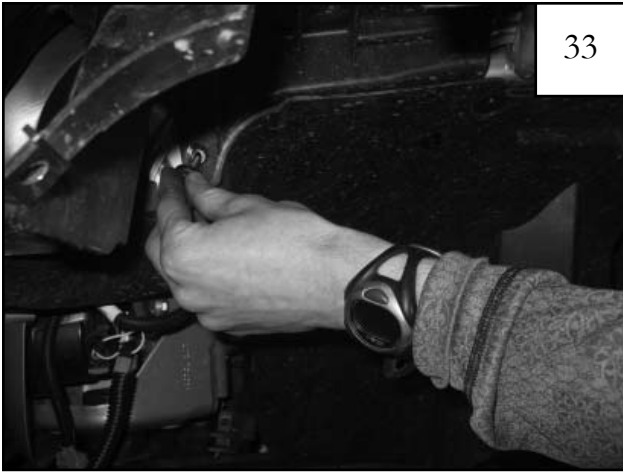
Reinstall the factory bolt at front of splash shield.
