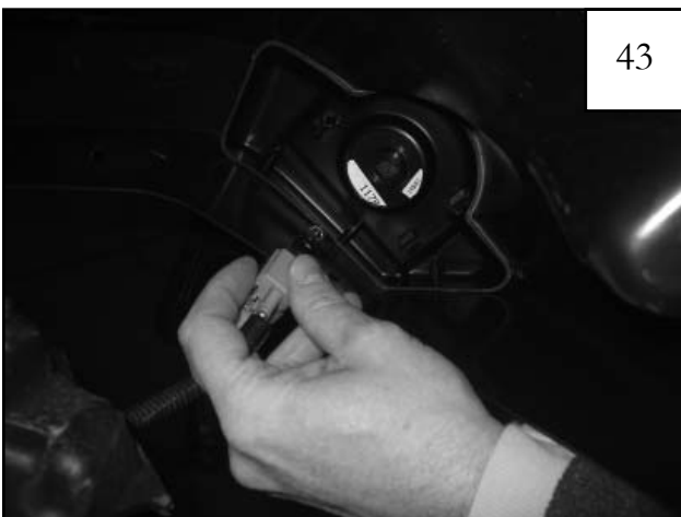
Reconnect light receptacle to light lens, then position Front Flare over Inner Flare Piece.
