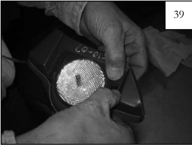
Press light bezel into light pocket inner piece, snapping tab into hole in light pocket inner piece.
