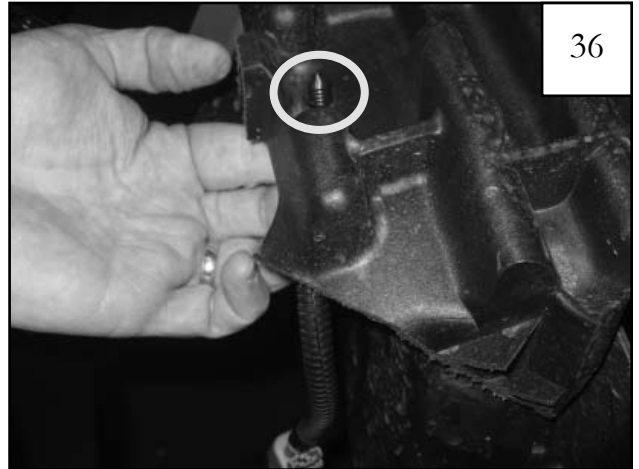
Reinstall Christmas tree clip in hole in factory Inner structure. Reconnect light cord to wire harness.
