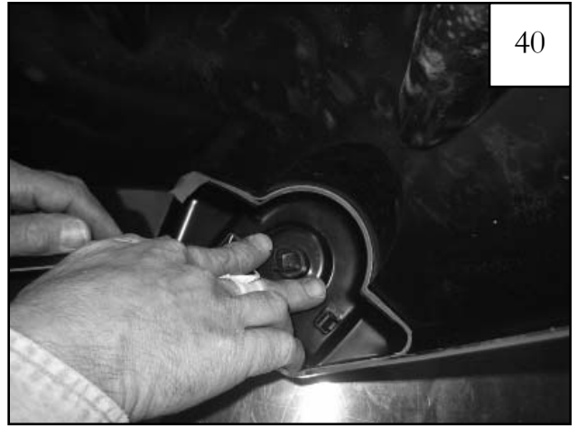
Place Light Pocket Inner Piece with light bezel into inside of Front Flare, aligning light lens with hole in flare. NOTE: Make sure tape liner is protruding from part for ease of liner removal.
