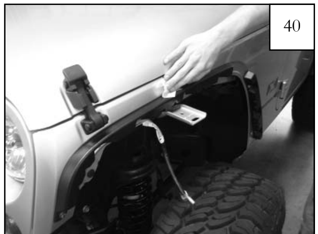
Use one supplied alcohol prep pad to clean the sheet metal above each inner piece in preparation to tape the edge trim to the sheet metal. This must be done for proper flare installation.
