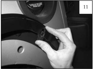
Install supplied "U" Nut, with the thread side in, over holes in Inner Flare Piece (8 places).
