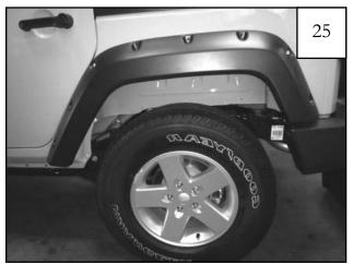
Ensure fit, and tighten all screws
