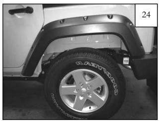
Ensure fit, and tighten all screws
