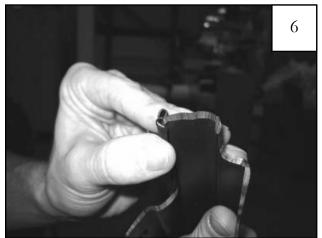
When positioning gimp on narrow end of rear, fold flat edge of gimp over the edge of the part. (Gimp will continue over entire length of part.)
