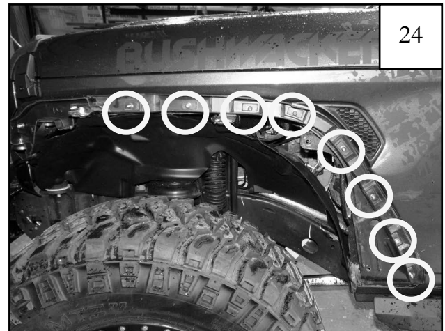
Step 3 Secure inner piece D2 with allen bolts and washers using the same procedure described in Step 22 and 23.
