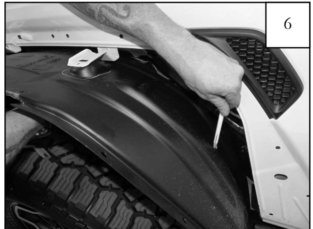
Using sheet metal as a guide, mark the rear portion of the splash shield with a grease pencil in preparation for trimming. The splash shield should be flush with the sheet metal after being trimmed. NOTE: If trimmed too little, flare won't fit; if trimmed to much, shield won't stay behind flare. Rear portion beneath vent may be left long.
