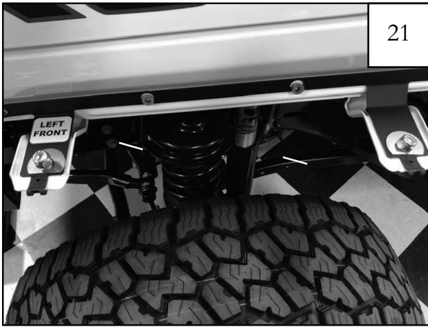
Support bracket flange properly attached to existing factory support in (2) locations.
