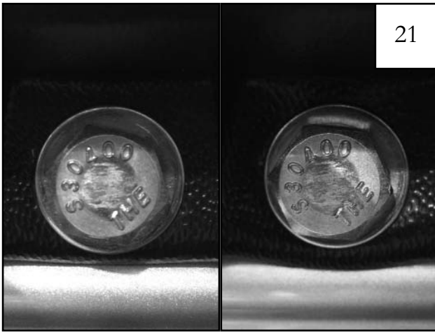
Bolt on left: Properly tightened; lower edge of inner piece runs straight Bolt on right: Overtightened; lower edge of inner piece bows down; if accidentally overtightened, remove inner piece completely before reinstalling
