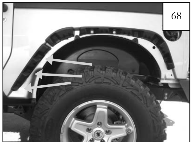
Secure inner piece D3 (and P3 for passenger side installation) to the sheet metal using the following 2 STEPS: Step 1 Position inner piece on fender, aligning with existing factory holes in sheet metal.
