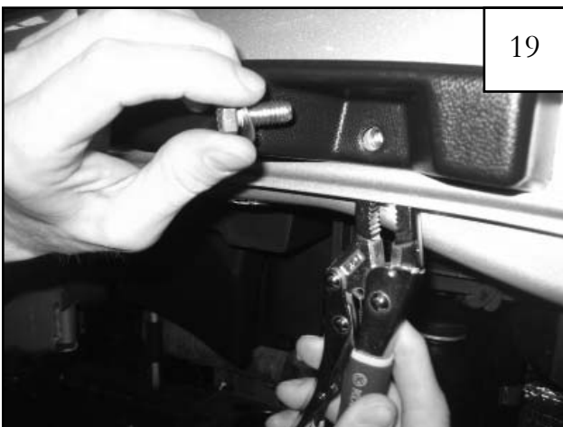
Step 3 For the rearward two mounting locations, use a vice grip to place the Nylok Nut on the back side of the bolt. Start the bolts but do not tighten.
