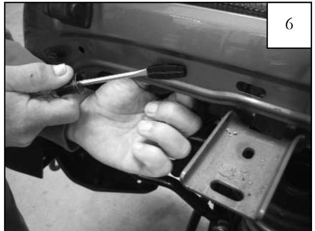
Using a pry tool or flat head screwdriver, remove any plastic clips still in fender.
