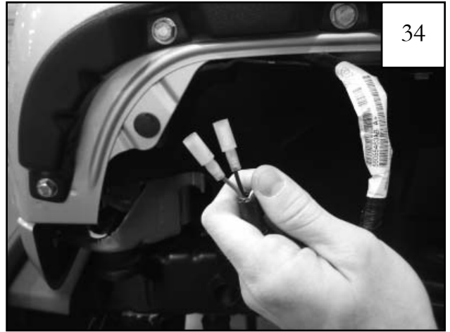
Install a Female Bullet Connector to the end of each factory side marker light wire and secure by pressing firmly with a wire crimp.
