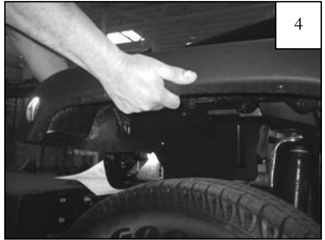
Starting at front of flare, pull firmly to release flare and splash shield from fender, working your way to the back. You will hear popping noises as clips release. It is okay. If clips break, they will be discarded.
