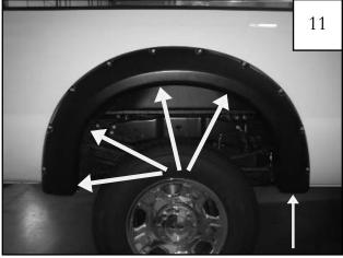
Ensuring proper flare placement, tighten all screws.
