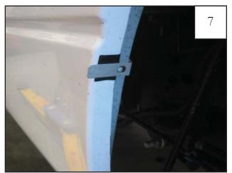
Install a Clip (CL1-0009) over each of the four Tabs (MT1-0014) placed on the sheet metal in Step 6.
