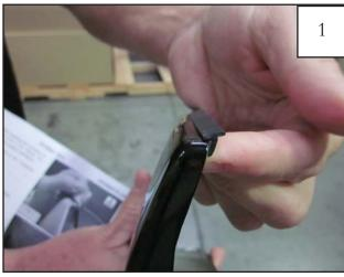
Peel two to three inches of red vinyl backing away from Edge Trim (GP1-0007) tape. Applying the adhesive side of the edge trim to the inner side of the flare, affix the edge trim to the top edge of the flare (the portion that comes in contact with the vehicle).
