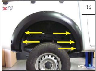
While holding Rear Flare onto vehicle using a #2 Phillips Screwdriver, start six (6) supplied Screws (SW1-0056) into flare and into clips installed in steps 13 & 14.
