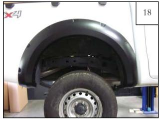
Tighten all screws. Rear flare installation complete.
