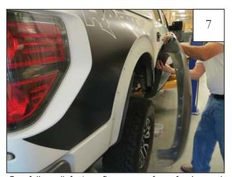
Carefully pull factory flare away from fender and remove. Using pliers, remove factory plastic clips. Clean the fender area.
