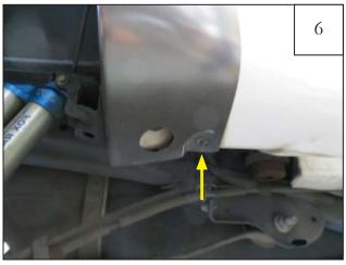
Use a 7/32 socket to remove the factory screw located at the front of the wheel well. Discard screw.
