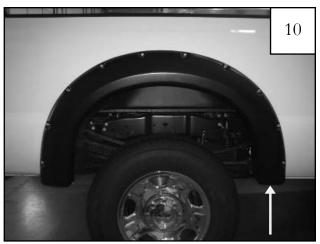
Place flare on fender and reinstall bolt removed in Step 5.
