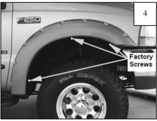
Remove three factory screws with a 7/32" socket wrench. Save for reinstallation. Position flare on fender. Apply moderate pressure to outside surface of flare and fasten to vehicle with three factory screws.
