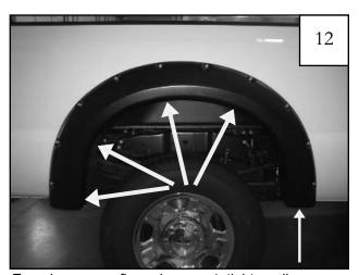
Ensuring proper flare placement, tighten all screws.
