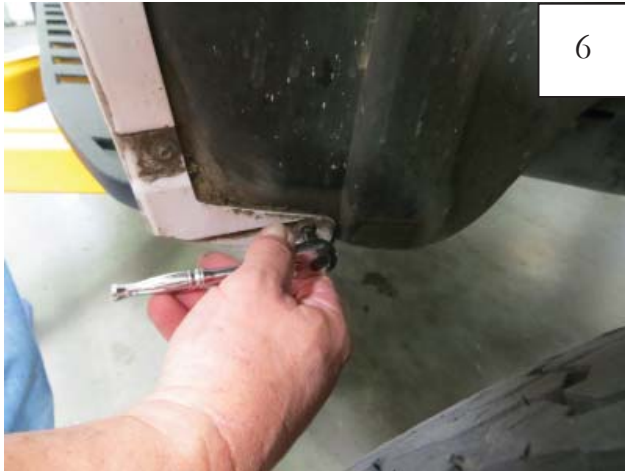
After removing factory flare, use a 7/32 socket to remove the factory screw located at the bottom rear of the wheel well. Retain screw for re-installation.
