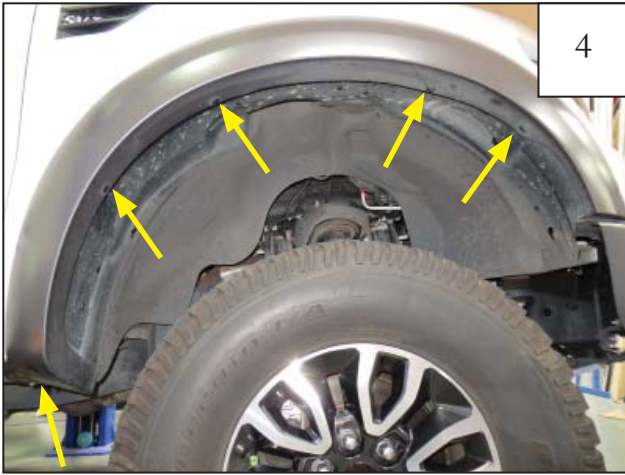
Using a pry tool, remove 5 retainers from the factory flare. Discard factory retainers.
