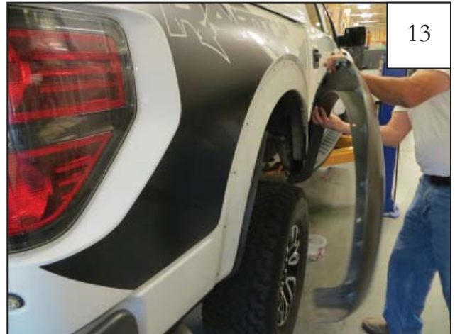
Carefully pull factory flare away from fender and remove. Using pliers, remove factory plastic clips. Clean the fender area.
