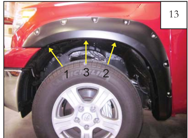
Start Screw (SW1-0050) in location #1 first, then move to #2, and start in location #3 last.
