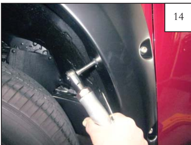
Start Screw (SW1-0036) through the three lower rear holes in flare and into factory holes in rear of wheel well.
