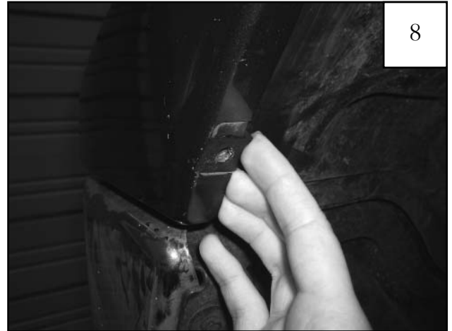
Slide a supplied "U" Clip over the fender lip, aligning with forward-most hole in fender. Note: For the Limited version, skip this step.
