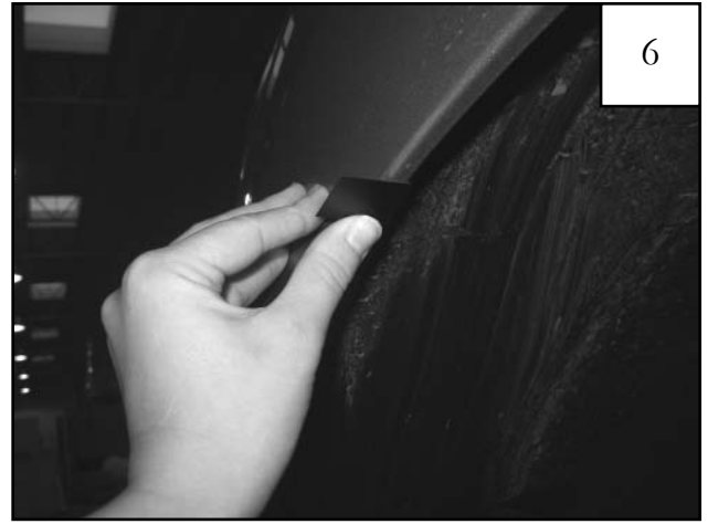
Remove flare from fender. Center a supplied Black Tab over each mark made in Step 4.
