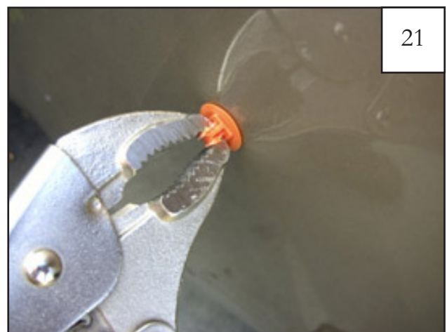
Remove three clips from fender using vise grips, pulling with a rocking motion. See step 22.
