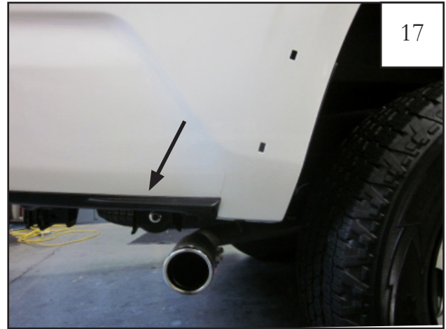
OPTIONAL: If there is no factory flare installed on the vehicle, you will need to remove the guard piece located at the rear of the bed or it will interfere with flare installation.
