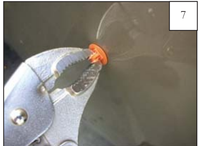
Remove three clips from fender using vise grips, pulling with a rocking motion. See step 8.
