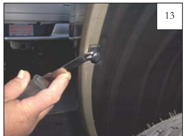
Remove plastic screw located at front of wheel well by turning clockwise 1/2 turn with a flat head screwdriver and prying out.
