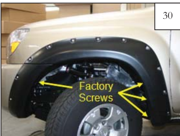
Reinstall four factory screws through holes in flare and into factory holes.
