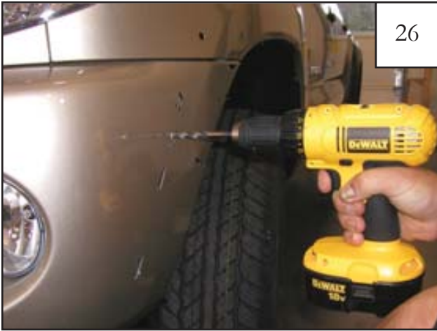
Remove fasteners installed in steps 23 - 24 and remove flare from fender. Drill at marked places with a 5/16" drill bit.
