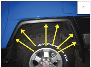
Using a 10mm socket, remove six bolts.
