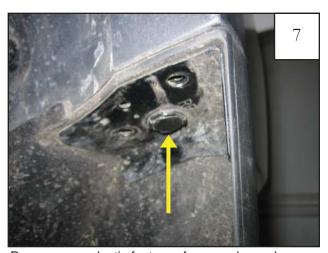
Remove one plastic fastener from mud guard.
