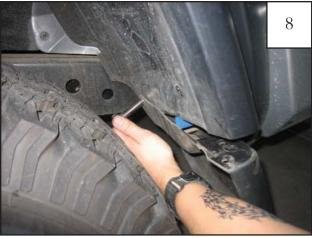
Remove bolt from mud guard located inside wheel well.
