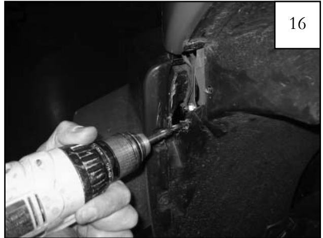
Remove Front Inner Piece, and drill two 5/16" holes on marks made in previous Step (2 places).
