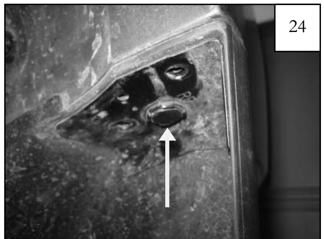
Remove one plastic fastener from mud guard.
