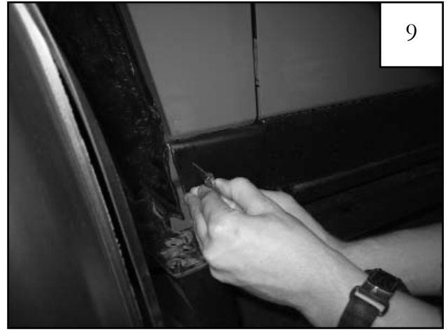
Trim an additional 3/4" from rocker, so that end of rocker is within confines of sheet metal. NOTE: The Flare will cover this area to 1/4" from the door seam.
