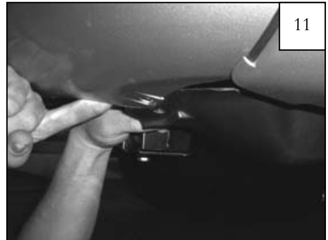
Pull down bumper cover and splash shield.
