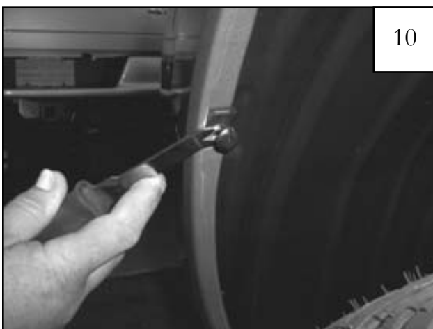
Remove plastic screw located at front of wheel well by turning clockwise 1/2 turn with a flat head screwdriver and prying out
