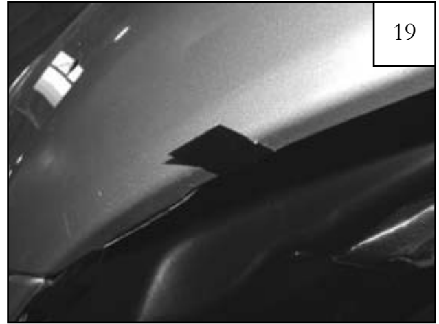
Remove flare from fender. Stick a supplied 1" Black Tab (MT1-0002) over marks made in step 17.
