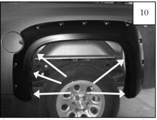
Start a supplied Screw (SW1-0050) through each of the remaining holes and into each Clip (CL1-0005) installed in step 8. If needed, use awl to locate holes.
