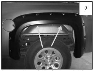
Reposition flare on fender. Start a supplied Screw (SW1-0058) through upper two hole locations and through each Clip (CL1-0022) installed in step 7. If needed, use awl to locate holes.
