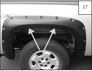
Reposition flare on fender. Start a supplied Screw (SW1-0058) through upper two hole locations and through each Clip (CL1-0022) installed in step 17. If needed, use awl to locate holes.
