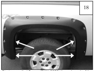
Start a supplied Screw (SW1-0050) through each of the remaining holes and into each Clip (CL1-0005) installed in step 16. If needed, use awl to locate holes.
