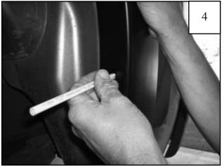
Holding flare in position on fender, use a grease pencil to mark five hole locations.
