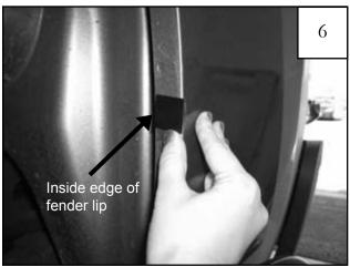
Center a supplied Tab (MT1-0002) over the marks made in step 4, aligning edge of tab with inside edge of fender lip (tab may extend over outside of fender).
