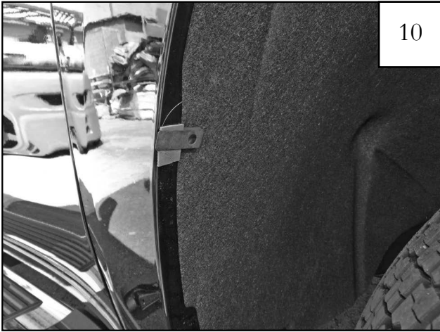
Install a supplied Clip (CL1-0009) over each Tab (MT1-0034).
