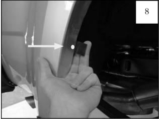
Wrap five supplied tabs (MT1-0034) around inner lip of sheet metal over the marked locations.
