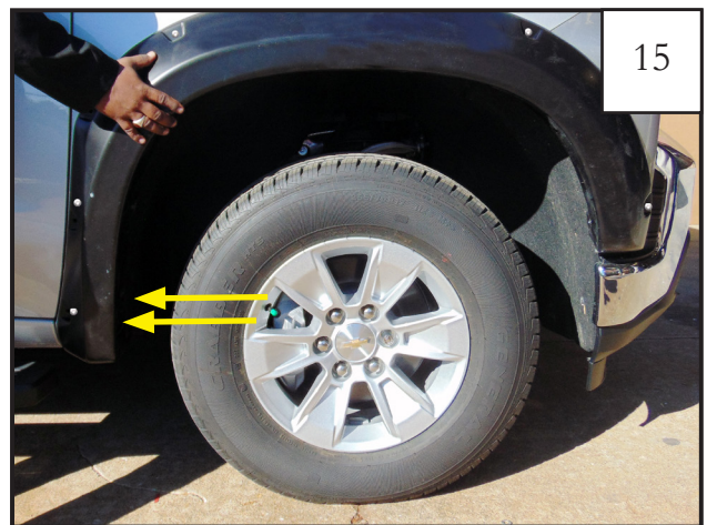
15 Re-install (2) factory screws (removed in Step 5) with a T15 bit. Do not tighten.
