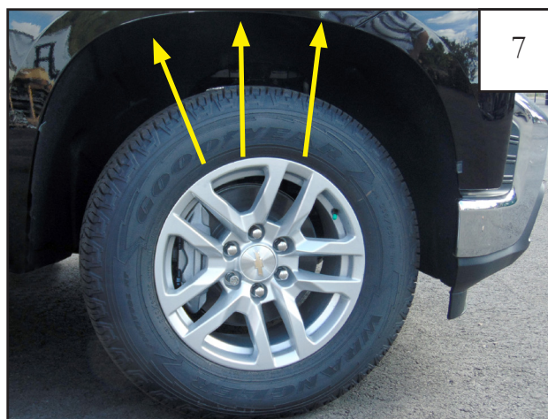
Remove (3) factory installed T15 screws from wheel well as shown above. These screws will be re-used to install the front flare.
