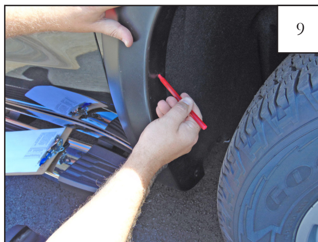
Use a grease pencil to mark the two locations of the holes indicated with the circles in Step 8. Remove flare from vehicle.
