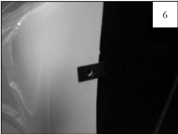
Install Clip (CL1-0011) over existing factory hole.
