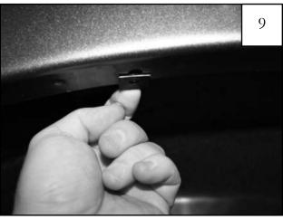
Install Clip (CL1-0022) over tabs and existing factory holes. There are two holes at the top center location. The hole for proper installation is the one toward the front of the vehicle. NOTE: The clip may fit over the lip loosely. This can be fixed by pinching the clip more tightly to the vehicle.
