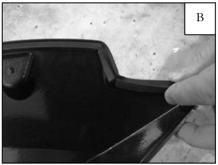
At the inward, right angle curve in the flare, cut a notch in the edge trim so when you along the part, the edge trim doesn't stretch.
