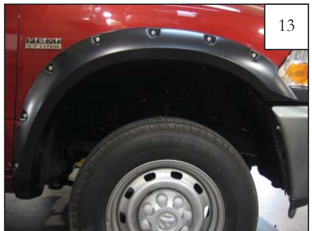
13 Completed front flare installation.
