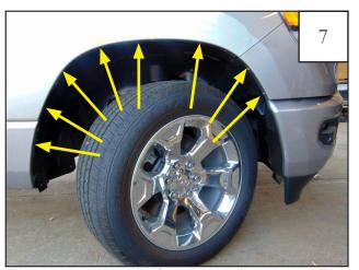
Remove and keep (8) factory installed screws. The remaing screws will be re-used to install the front flare.
