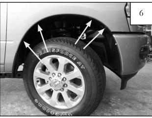
Remove and keep (4) factory installed screws. The screws will be re-used to install the front flare.
