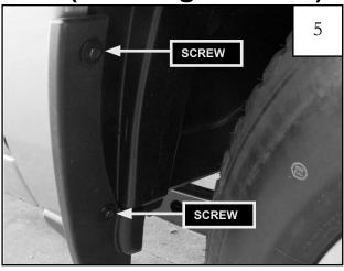
Remove (2) factory installed screws and remove mud flap from vehicle. Retain screws to be re-used to install the front flare.
