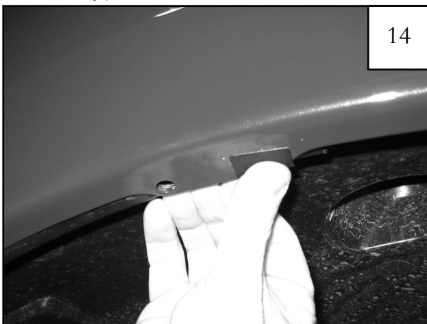
Install plastic tab over existing factory hole.
