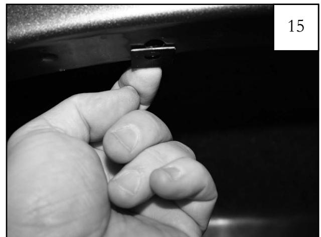
Install Clip (CL1-0022) over existing hole.
