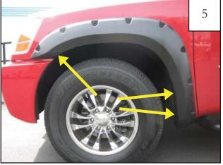
Position flare on fender. Line up the two lowest holes in flare with the factory holes and start the two factory screws. Line up the forwardmost hole in flare with the hole just above the bumper and start one factory screw. *Do not fully tighten screws.*
