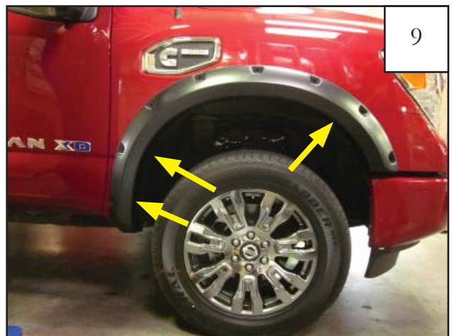
Position flare on fender. Line up holes in flare with the factory holes and start the two 3 supplied screws (SW1-0049) where indicated in picture. Do not fully tighten screws.
