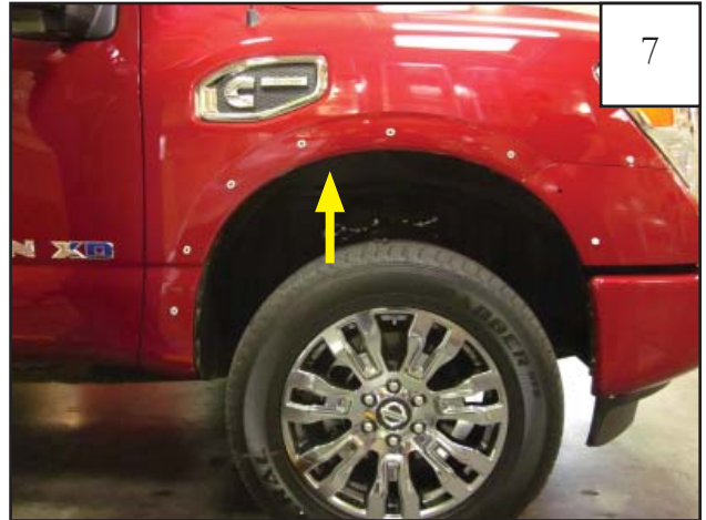
Using a #2 Phillips Screwdriver, remove factory screw from wheel well.
