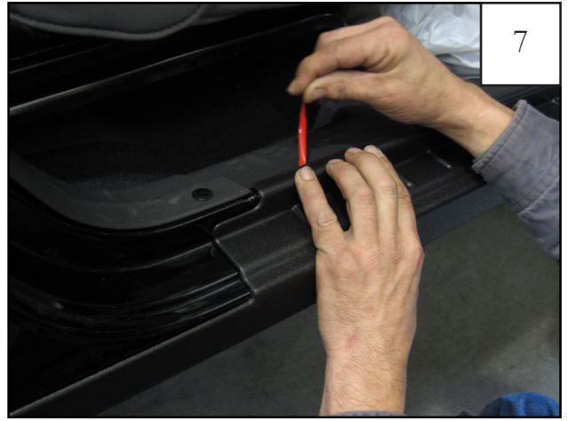
Pull 1/4" tape liner tab 2. NOTE: Refer to step 1 for additional tape tab identification.
